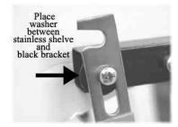
**STEP 3** Place one (D) long screw from the outside of the bracket through the sliding hole of the shelve hinge. The screw must be placed in from the outer part of the bracket. Make sure that you insert the long screw into the copper ring spacer before inserting into shelve hinge. Repeat the same on the other bracket hole. Secure the screws with a nut and black washer (in between shelve and bracket) on the top screw and a nut on the bottom screw.
