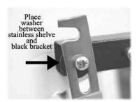
**STEP 3** Place one (D) long screw from the outside of the bracket through the sliding hole of the shelve hinge. The screw must be placed in from the outer part of the bracket. Make sure that you insert the long screw into the copper ring spacer before inserting into shelve hinge. Repeat the same on the other bracket hole. Secure the screws with a nut and black washer (in between shelve and bracket) on the top screw and a nut on the bottom screw.
