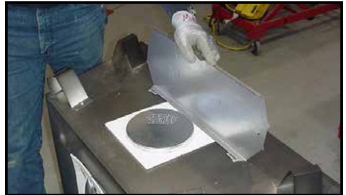
Figure 6.3 Rotate the top heat shield to the vertical position as shown above. The heat shield must remain in the vertical position.
