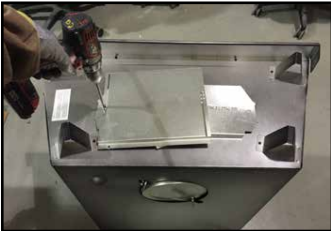
Figure 6.1 For top vent, remove the screw holding the elbow heat shield in place.
