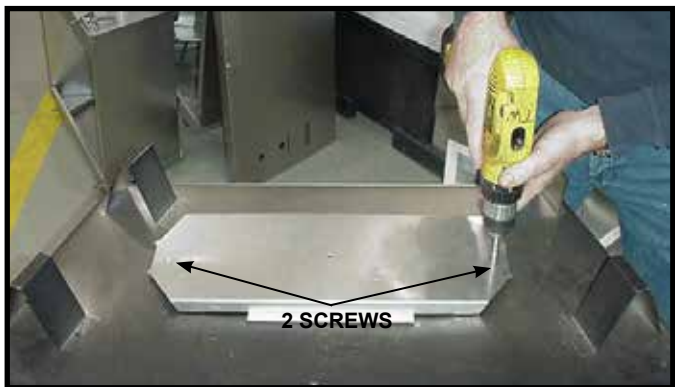
Figure 6.2 Remove the two screws holding the top heat shield in place.
