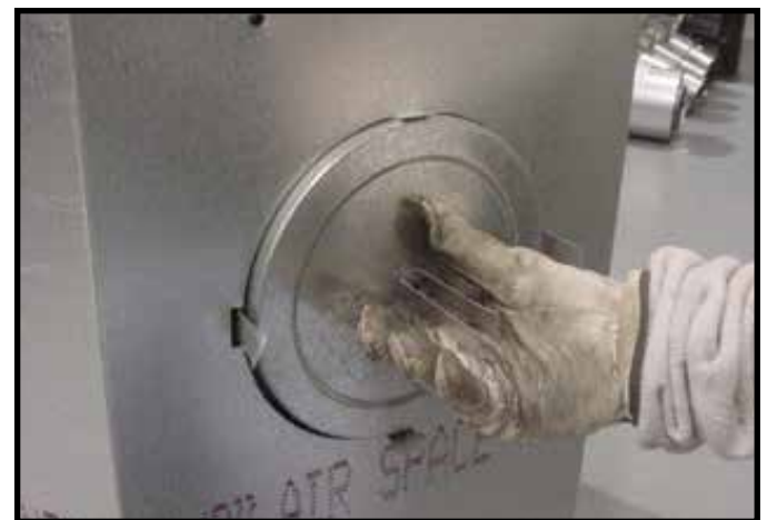
Figure 6.11 Fold the center parts of the retaining band out and use to remove the seal cap.
