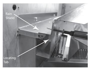
4. Lay bead of high temperature silicone in the channel between TRAP-VSS and cap rain shield to prevent water drainage between TRAP-VSS and rain shield.
