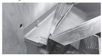
5. Apply bead of high temperature silicone on bottom surface of TRAP-VSS. Position the TRAP-VSS onto cap as shown and attach with (3) screws provided. Clean excess silicone as needed.
