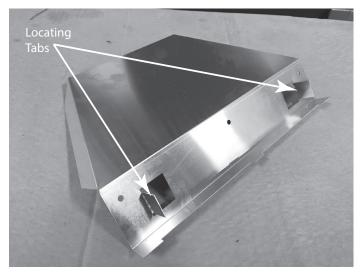
3. Position the TRAP-VSS onto existing cap as shown, and attached with (3) three screws provided. Make sure locating tabs are up against bottom edge of rain shield.
