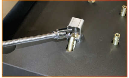
Photo L1: Lighting Jet Nearest Thermocouple
