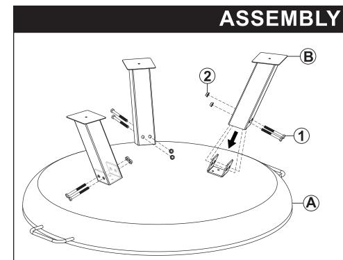
Align the mounting holes of one Leg (B) over the brackets on the bottom of Fire Bowl (A) and firmly secure using two M6x60mm Bolts (1) and two Flange Nuts (2).
