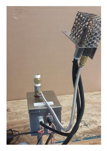
Step 6: Install the Pilot Burner Assembly as shown at right
