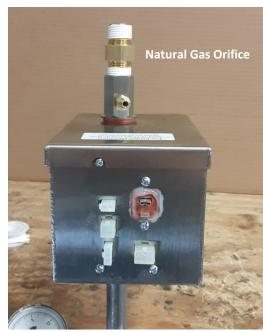
Step 5: Plug the Battery Pack and Control Panel into the receptacles on the front of the Ignition Control Box.
