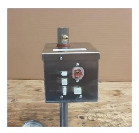
Step 4: Install the Brass Natural Gas orifice in the outlet of the Ignition Control Box.
