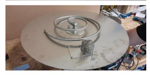
Complete the Install by adding the Lava Rock Media. When the media is installed correctly you should not be able to see the Pilot Burner unless you look very carefully as you see in the photo at right.
