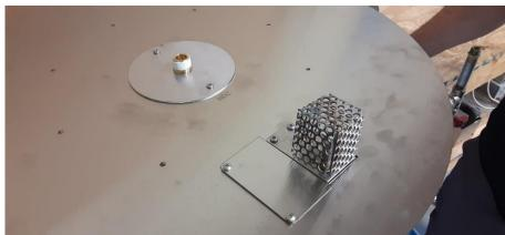
Step 9: Install the Spiral Burner as shown in the photo at right.
