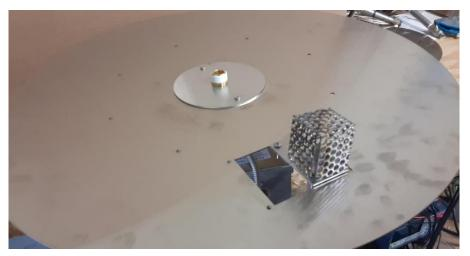
Step 8: There is a rectangular shaped plate should have been included with the battery system. Install the plate in the opening to the left side of the Pilot Burner as shown in the photo at right.
