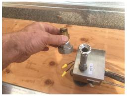
10. Install the Burner Pan. You will need to line up the Pilot Burner with the Opening for the Pilot Burner in the Burner Pan as shown in the photo at right.
