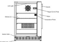
1. Position the unit to allow free air flow through the front grille.
